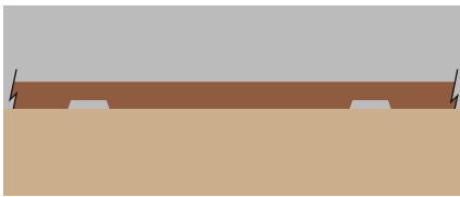
OPTIONAL PORTED BATTEN: MIN 1/2" WIDE 1/4" DEEP DRAINAGE PORT MINIMUM OF 2 FT. ON CENTER
