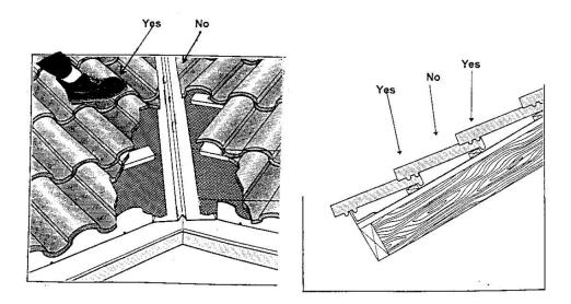
It is also recommended to stay away from hips or valleys to avoid breaking cut tiles that would be more difficult to replace. The exception to this would be in situations where the hips and ridges are bedded in mortar or foam, in which case, they may be preferred walking paths. Valleys may also be access paths if the tiles are cut away from the center of the valley wide enough to allow foot traffic on the metal valley flashing.
